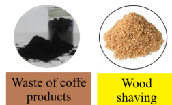
As a raw material in the production of activated carbon [9], as an indicative example, the use of coffee grounds waste with a fraction from 0.1 mm up to 1 mm is proposed. From waste of wood chips or shavings, it is proposed to use a large or small chip or shaving of sizes from 5 mm up to 20 mm.
